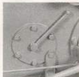
P.T.O. Lever in engaged position.
