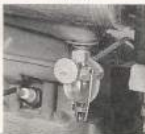
Fuel Valve and Sediment Bowl.
